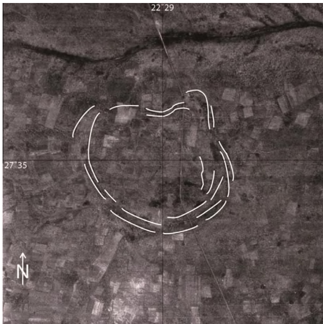
Fig. 27. Aerial photograph of the Kgagodi crater area in southeastern Botswana. The lines indicate the rough location of generally poor suboutcrop of the crater rim. The drill core that provided the proof of the impact origin for this geophysically recognized structure was obtained some 400 m inside of the northeastern rim.
