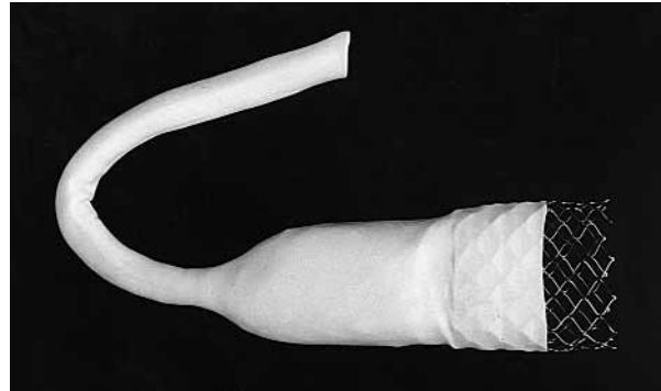
Fig 1. All patients recruited into the study underwent endovascular repair through the use of a handmade device composed of a balloon expandable Palmaz stent sutured to tapered PTFE graft.
