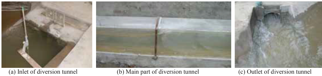
Fig.4 Flow model of diversion tunnel’s hydraulic model test for Gongguoqiao hydropower station (Q=3850m 3 /s)
