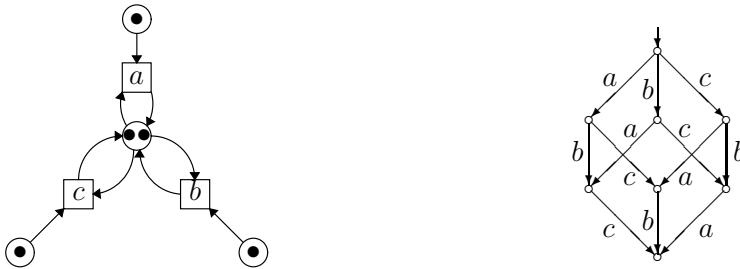
Fig. 10. A 2-out-of-3 semaphore , represented as a Petri net and as a higher dimensional automaton. In the latter, all six squares are supposed to be filled in, but the interior of the cube is not. Up to history preserving bisimulation equivalence this system cannot be represented as an automaton under the concurrent interpretation, because, due to the filled-in squares, the cube shape is unavoidable, and interior of the cube would by default be understood to be filled in. Hence the system can also not be represented as a pure Petri net.
