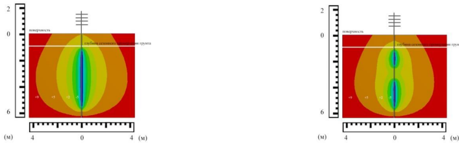
Experimental ground temperature field around TK 32 / 6M5 A-01 with the duration of the active period 180 days.
