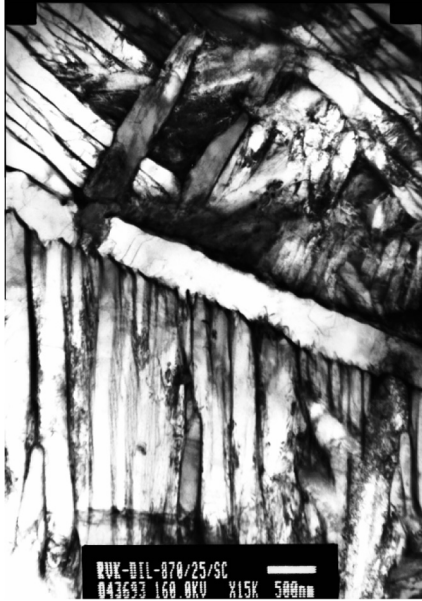
Fig. 1. Typical Widmanstätten plates were found in Zr–2.5Nb alloy [6].
