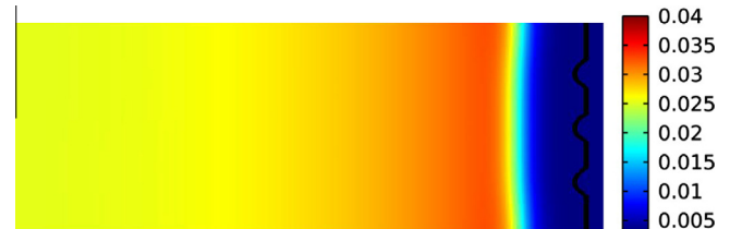
Fig. 9. Distribution of concentration field (mole fraction of Nb) during development of allotriomorphs \alpha from the protrusions of grain boundary \alpha at 1054 K. The black line denotes the initial position of the interface. The domain size is 2.80 \times 1 \mu\text{m} .
