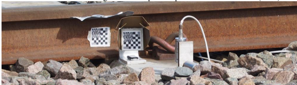
Figure 3: Sleeper end with DIC targets on sleeper and rail and a pair of horizontal and vertical geophones.
