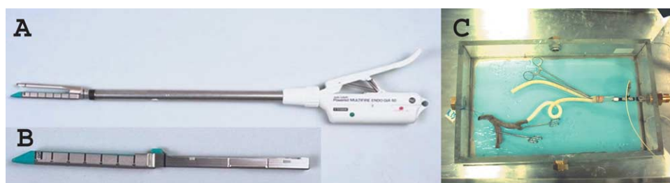
Fig. 1. Material: (A) multifire powered EndoGIA 60 ® (Tyco Healthcare, Norwalk, Connecticut, USA). (B) 4.8 mm staples for EndoGIA 60. (C) View of the hydrodynamic bench used for the experimental study.
