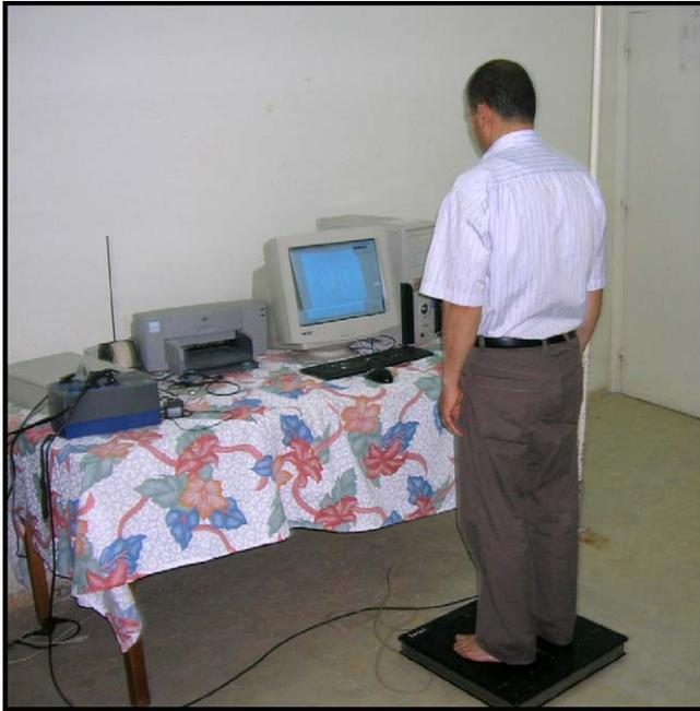
Fig. 1. Force platform for the assessment of static balance.
