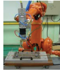
(b) Laser optic and welding robot
