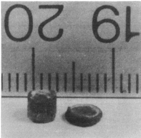
FIG. 63. Nanocrystalline \text{TiO}_2 -sample before and after compression at 810^\circ\text{C} for 15 hr with a stress of 40 MPa. The initial crystal size was about 40 nm. (388)
