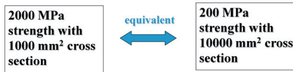
Fig. 6. Comparison of high and low strength/stiffness materials.
