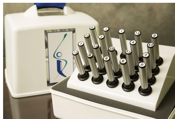
Fig. 3 The Snap and Sniff® Threshold Test. This modern test allows for rapid and reliable determinations of detection thresholds. Concentrations of phenyl ethyl alcohol, ranging from 10^{-2} to 10^{-9} \log vol/vol in half-log concentration steps are commonly employed, along with blanks for forced-choice testing. Photo courtesy of Sensonics International, Haddon Hts., NJ 08035, USA. Copyright© 2015, Sensonics International.
