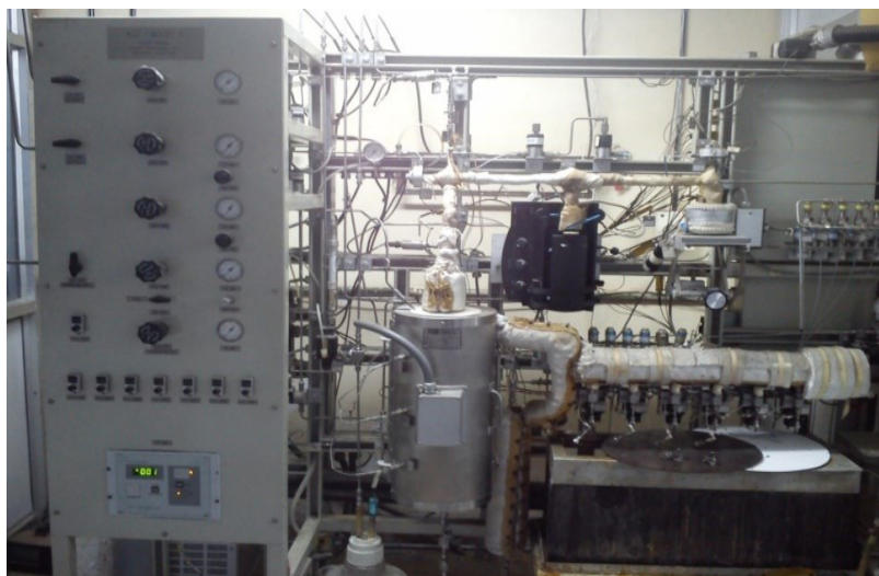
Fig. 2 Experimental setup for fluid catalytic cracking (ACE-R) unit
