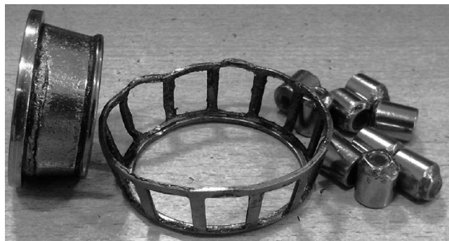
Fig. 6. As illustrated in the schematic diagram (Fig. 5), damage at roller tip and deep groove on the cone were observed on the premature failed bearing.
