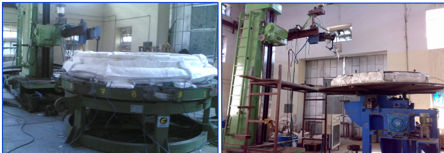
Figure 6 Seal ring hardfacing in the shop
