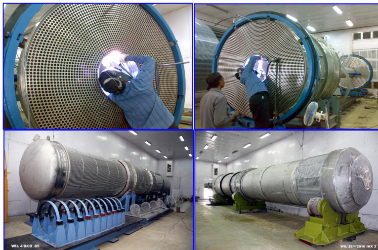
Figure 4: Fabrication of Intermediate Heat Exchanger
