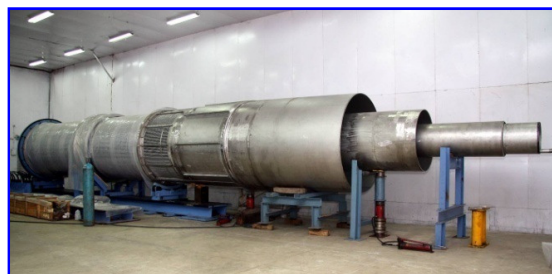
Figure 3: Shell fabrication stage of Intermediate Heat Exchanger
