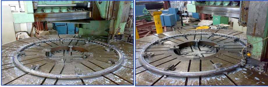
Figure 10 Seal ring machining in the shop
