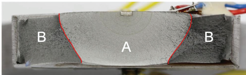
Fig. 7. Fracture surface with beach marks.
