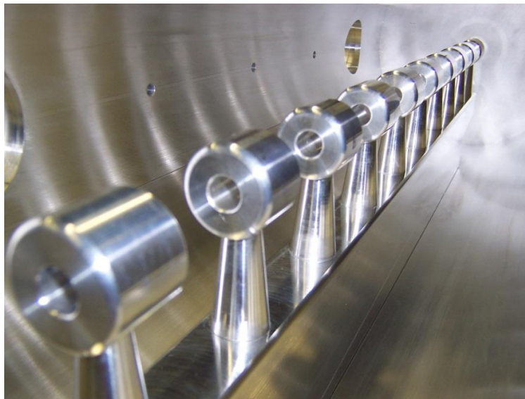
Fig. 7. Drift tubes installed on the bottom part of the IH cold model. The top part is not yet inserted here.
