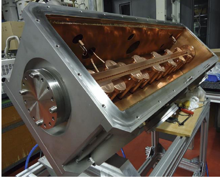
Fig. 4. Fermilab 201.25-MHz 4-rod RFQ for 60-mA H^+ beam (2012).
