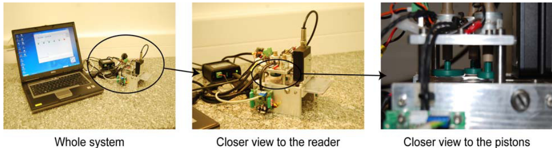
Fig.2 Views of the prototype. Left: a general view with the driving computer. Middle: a closer view of the reader. Right: pistons used to drive the fluids.
