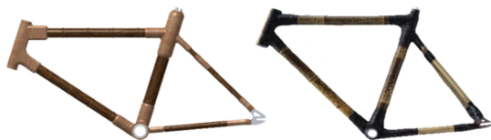
Fig. 4. Bamboo frame CAD model (left) and manufactured frame (right)
