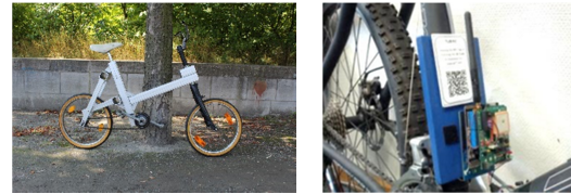
Fig. 5. Modular “lego” bicycle build out of standardized aluminium profiles (left) and sensor equipped bicycle (right)
