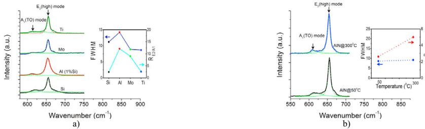
Fig. 3. Raman spectra of AlN thin-films deposited (a) on different seed layers and (b) on Ti at room temperature and 300 °C.
