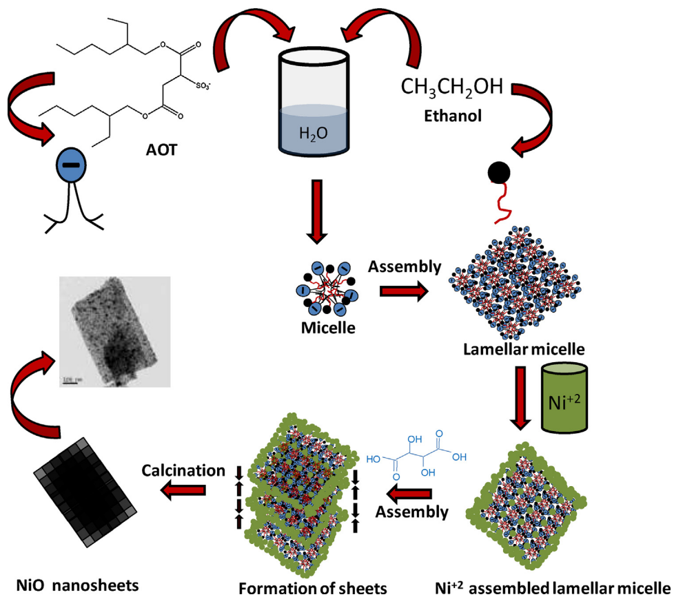
Fig. 5. Schematic illustration for the formation of NiO nano-sheets.
