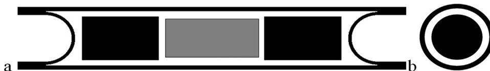
Fig. 3 – Cross sections of TheraSeed 200: (a) longitudinal cross section and (b) transverse cross section (ID: 2200).
