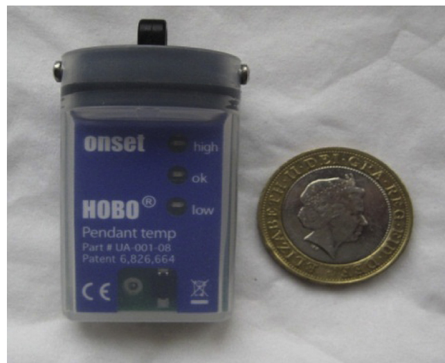
Fig. 1. HOBO pendant temperature loggers used for indoor temperature monitoring.
