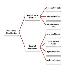
Fig. 2: Data Fusion Classifications within WSNs
