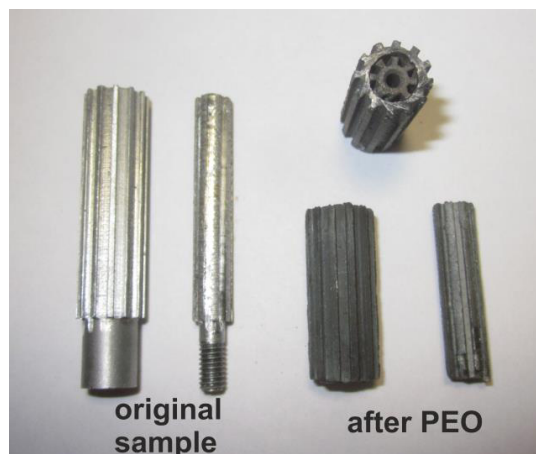
Fig. 1. Original catalyst carrier samples and the catalysts obtained by plasma electrolytic oxidation and palladium activation (after PEO).
