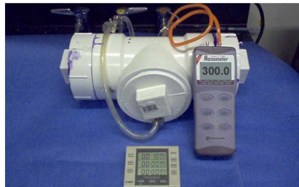
Fig 1. Custom pressure chamber designed to expose standard tissue culture plates to hyperbaric pressure.
