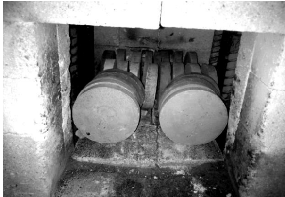
Fig. 3. Circular bricks placed in oven.
