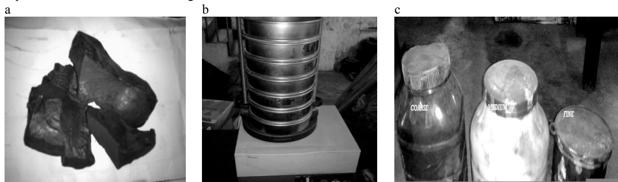
Fig. 1. (a) Hard coal pieces, (b) sieve analyzer, (c) Coarse, medium and fine coal powders collected after ball milling and sieve analysis.
