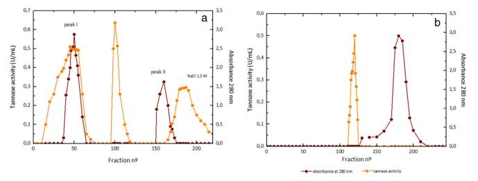
Fig. 2. (a) DEAE-Cellulose and (b) Sepharose CL-6B chromatographic profiles for tannase produced by the fungus A. carbonarius.
