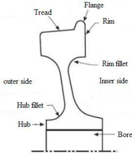
Figure 1. Designations of each part of a solid railway wheel.
