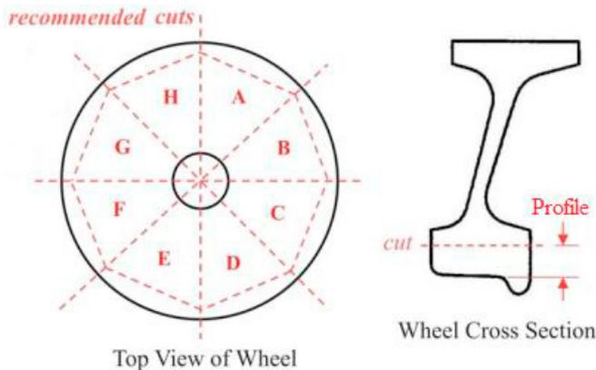
Figure 2. Front view and railway wheel profile with cut recommendation.
