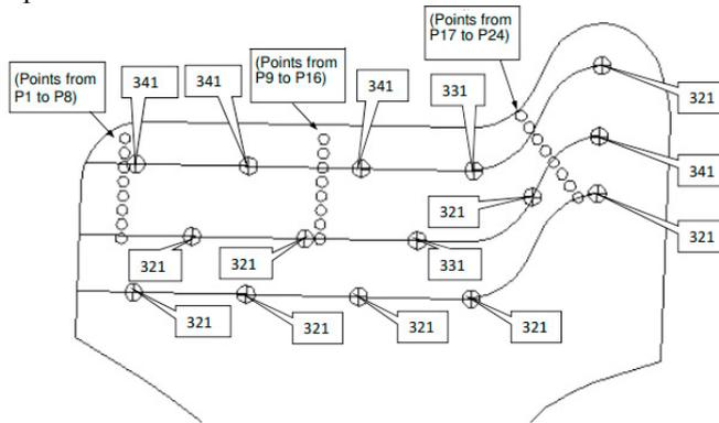
Figure 5. Brinell hardness results and Rockwell C Hardness points of the rim profile of the Railway Wheel.
