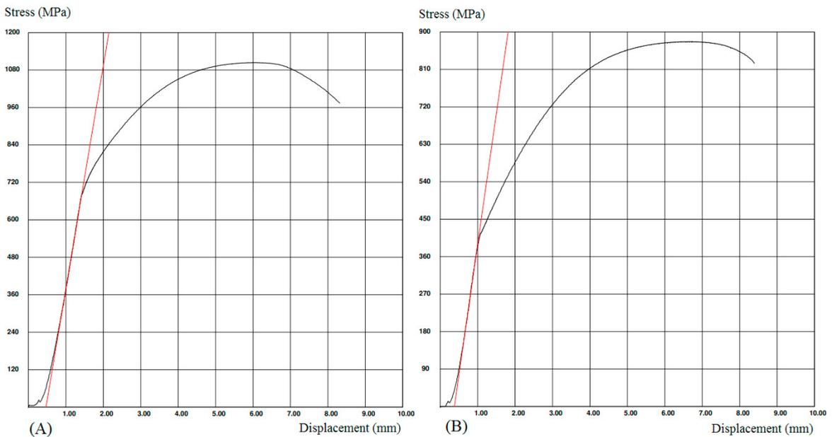
Figure 6. Tensile testing result - (A) Rim and (B) Wheel Disk Stress (MPa) versus Displacement (mm)
