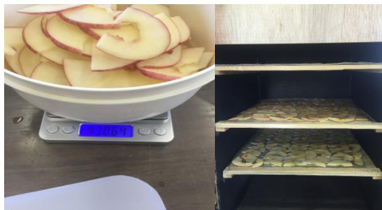
Fig. 1. Weighing a portion of product (left) and drying product inside the drying chamber (right).
