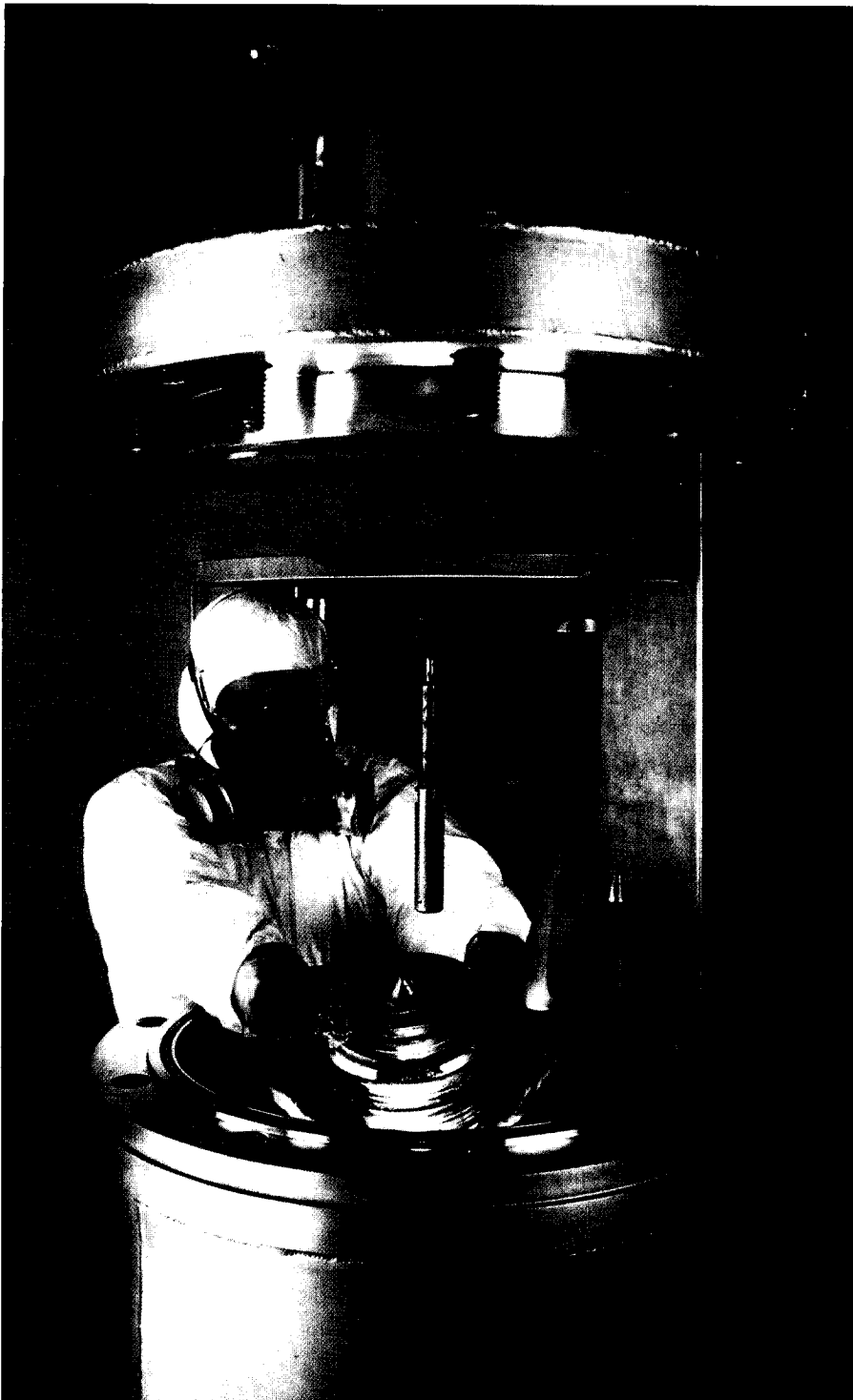
SG 15/25 HPLEC crystal growth system and 150mm diameter GaAs Ingot.
