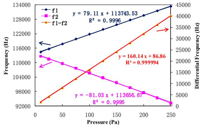
Fig. 7. The frequency responds of the resonators under applied pressure.
