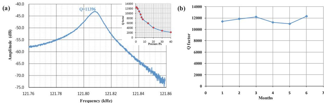
Fig. 6. (a) The Q-factor of the micro fabricated sensor is more than 10000, which indicates the vacuum achieved in the micro chamber is less than 5Pa. (b) The constant Q-factor in the past 6 months indicates the reliability of vacuum packaging and interconnection.
