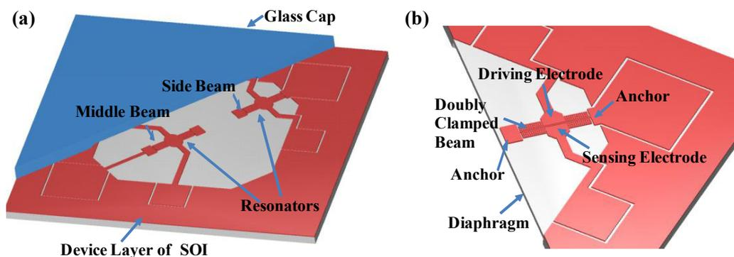
Fig. 1. (a) Top view of the proposed sensor with dual resonators packaged; (b) enlarged view of the resonator.
