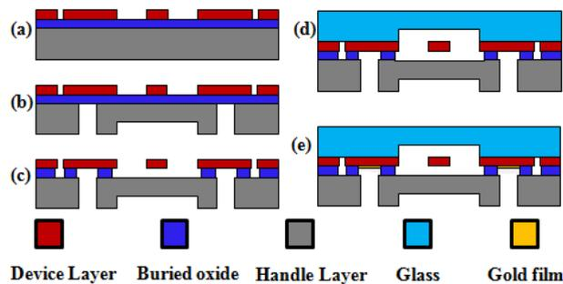
Fig. 2. The simplified fabrication flows of the proposed resonant pressure sensor.
