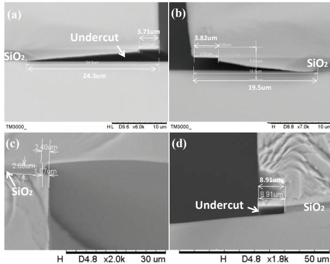
Fig. 5. The etching results with Vapor HF. (a) and (b) are the SEM image of removing SiO<sub>2</sub> in via holes without water removal; (c) is the SEM image of removing SiO<sub>2</sub> in via holes with the 2-step cycle process; (d) shows the release of the resonator using the 2-step cycle process, the undercut on the anchor was limited in 10 μm.
