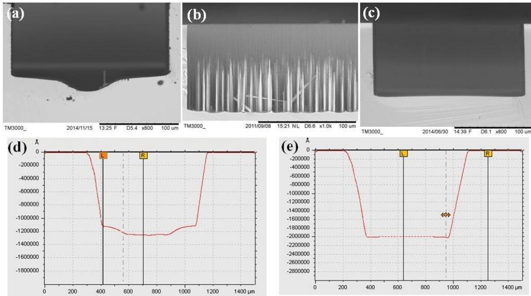
Fig. 3. The etching results with different masks. (a) and (d) Z4620 (4  $\mu\text{m}$ ); (b) Al (100 nm); (c) and (e) ZnO (100 nm).
