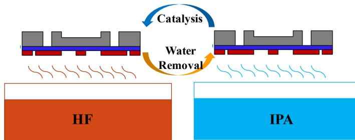
Fig. 4. Releasing the resonators with the proposed the 2-step cycle processes
