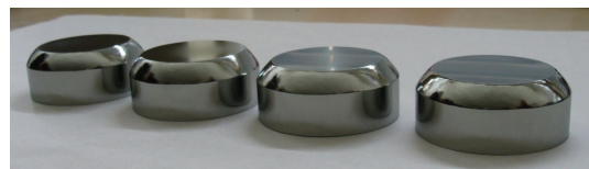
Fig. 5 Ultra-pure Ge crystals of the GEMMA experiment.
