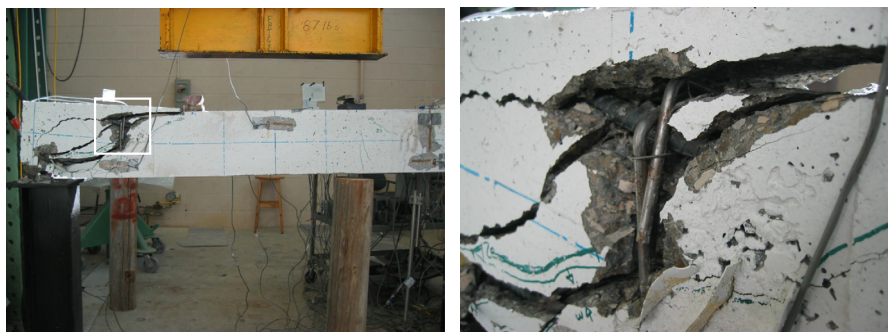
Figure 13 Untied stirrup in arch failure mode.
