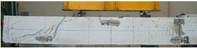
Figure 8 Crack patterns of RC beam with pre-cracks at different locations and orientations.
