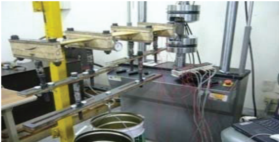
Fig. 9 Multi-point loading test
