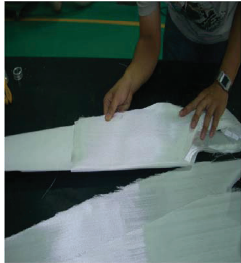
Fig. 3 Core wrapped by glass fabric
