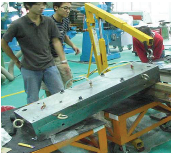
Fig.4 Steel mold for VRTM
