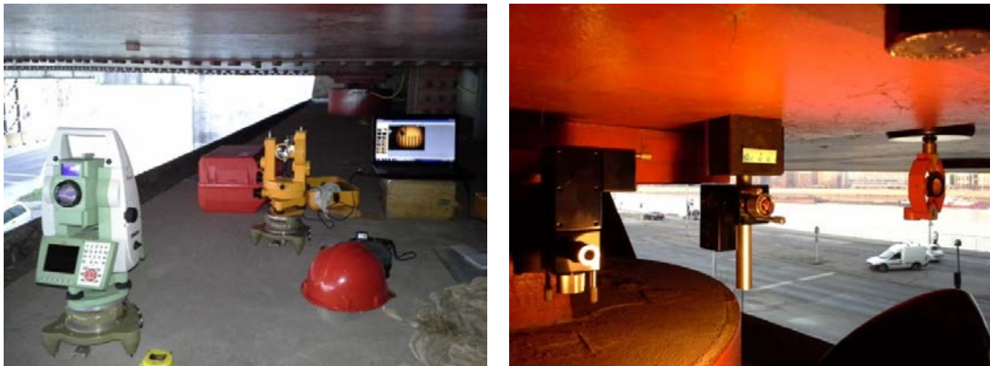
Fig. 8. Layout of the measuring station: a) theodolite and digital camera, b) laser interferometer.
