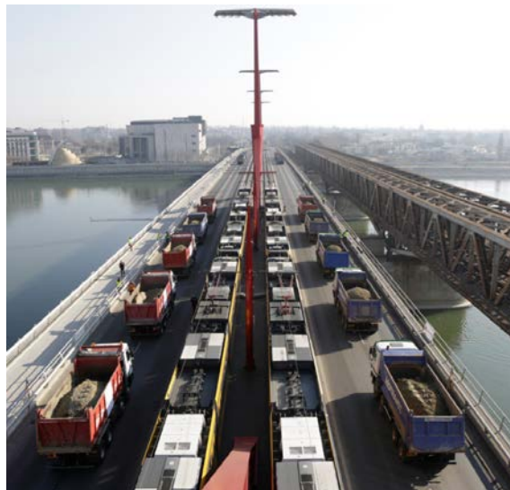
Fig. 2. Typical loading situation during the loading test using 12 trucks and 4 trams in one span.
