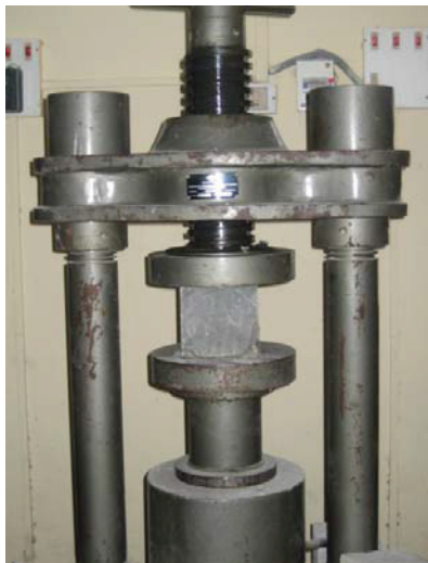
Figure 3: Plate 1 Test for Compressive Strength
