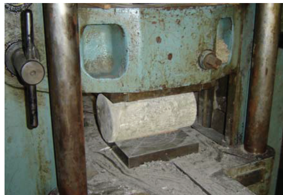
Figure 4: Plate 2 Test for Splitting Tensile Strength
