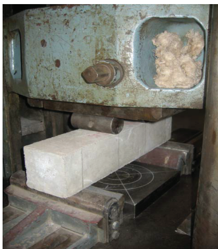
Plate 3 Test for Flexural Strength of Concrete
