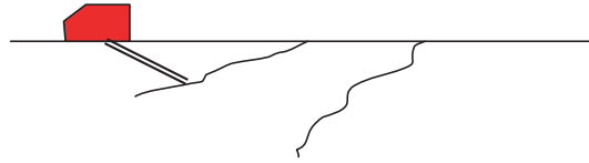
Fig. 1. Shallow crack shadowing.
