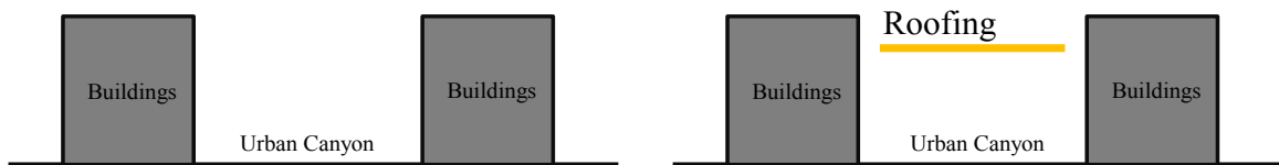
Fig. 1. The two situations considered: an urban canyon without canopy shading, and a street canyon with a tent positioned at rooftop level.
