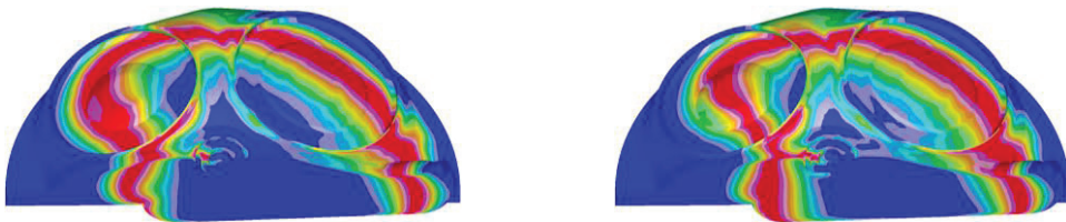
Fig. 9. flame front @ 740°CA: fuel only (left) and water/fuel (right).
