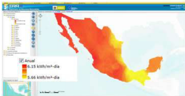
Figure 4. Average annual horizontal insolation for Mexico, kWh / m 2 / day. Taken from Renewable Resource Explorer of IIE (2013).
