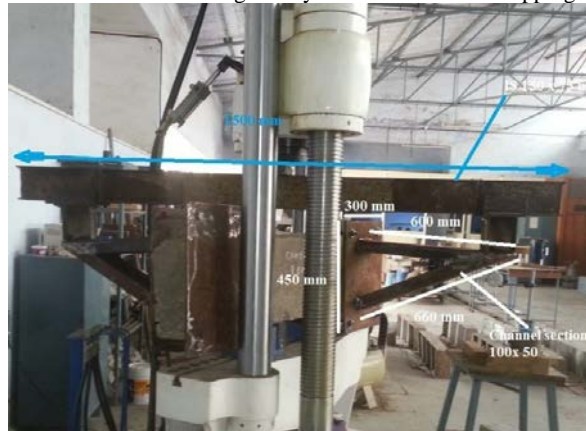
Fig 5 Test beam fixed to torsion assembly
