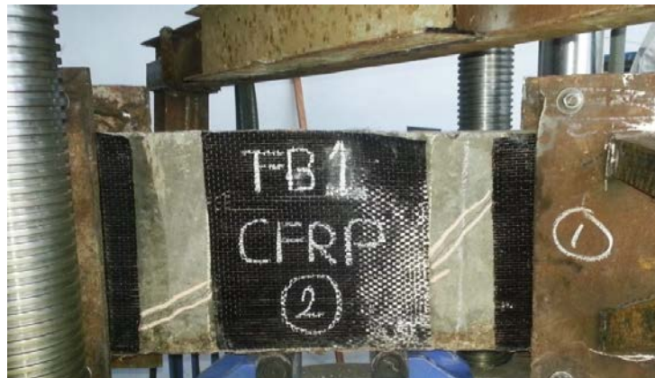
Fig 7 CFRP bonded RC beam (CFB1) before testing
