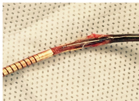
Figure 2 Insulation breach in the extracted St Jude Medical Durata lead near the distal defibrillation coil.
