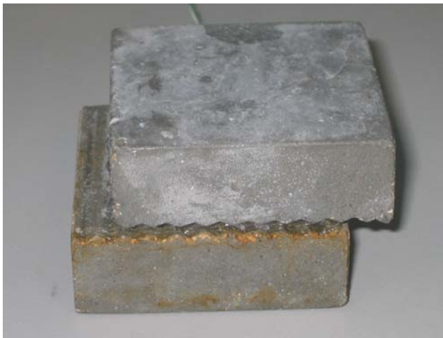
Figure 4. Sandwich sample after a constant stress test with normal stress = 207 kPa.
