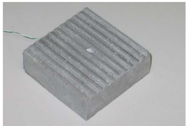
Figure 2. Concrete block with cast saw-tooth surface; the small cavity in the center holds the tip of the thermocouple.
