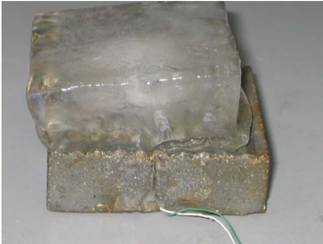
Figure 12. Shear deformation of a concrete-ice sample after a constant strain test with normal stress = 490 kPa.
