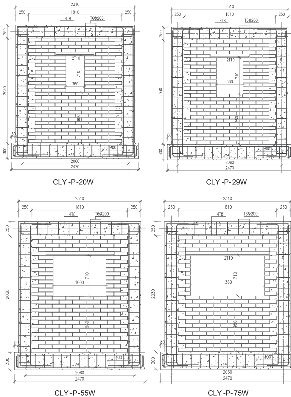
Fig. 13 Tested CM walls.
