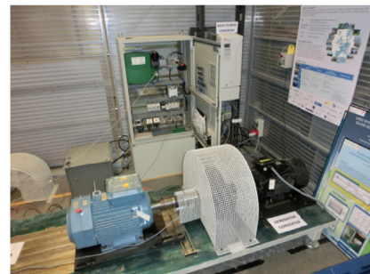
Fig. 7. Configuration used for the hardware-in-the-loop validation tests.
