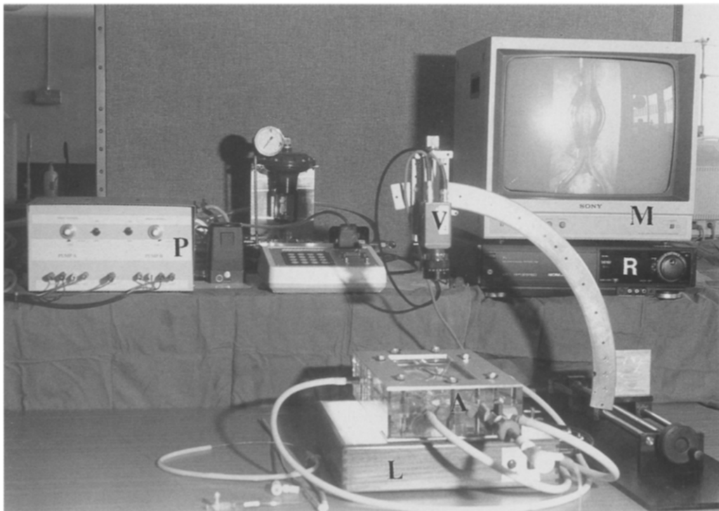
Fig. 3. Photograph of the uncovered training simulator showing the video camera (V) supported by an adjustable C-arm and movable gantry, AAA model (A), light-box (L), display monitor (M), video recorder (R) and pulsatile pump system (P). The computer which performs the video image acquisition and processing for mock aortograms and road-mapping is not shown.
