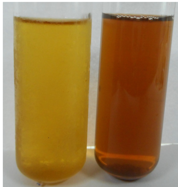
Fig. 2. Photograph showing the color change pattern during nanoparticle synthesis; (A) crude fruit extract of N. nimmoniana (50 mg/mL); (B) AgNO 3 with the fruit extract forming AgNPs after 1 h of incubation.
