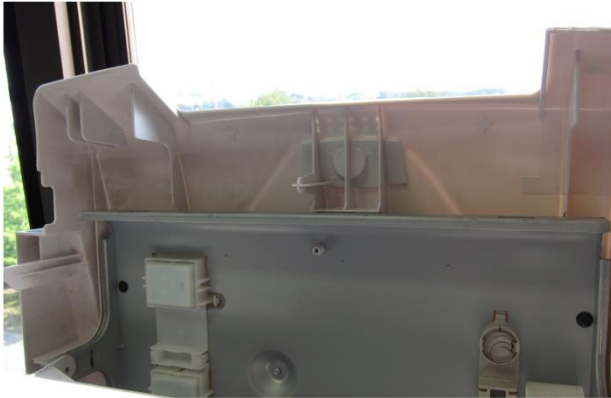
Figure 2. Rib features placed on a plastic part.
